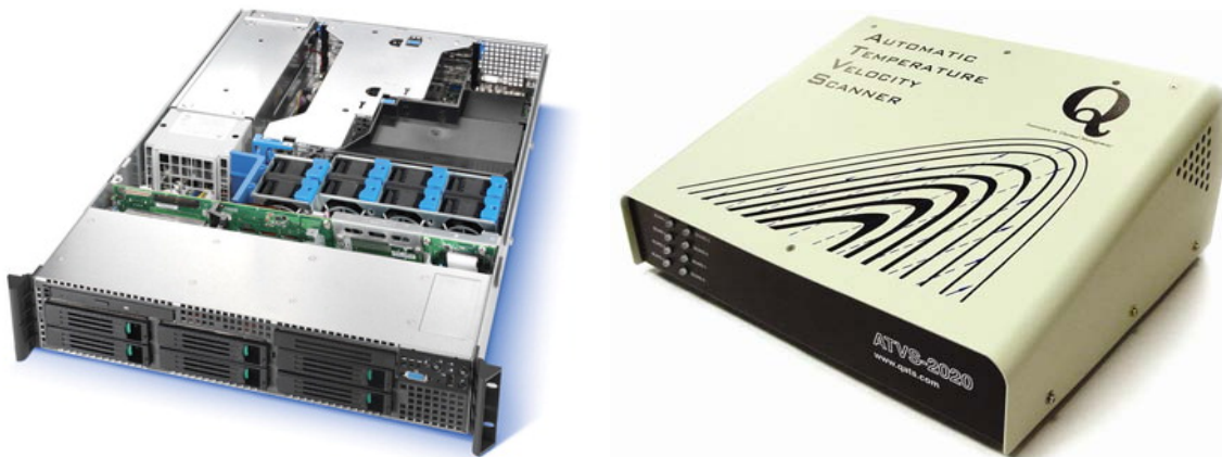
Figure 3. An Intel SR2400 server chassis (Left) and an ATS ATVS-2020 automatic temperature and velocity scanner (Right) were used to test the ATS-725 heat sink performance on a WANic 3860 card
